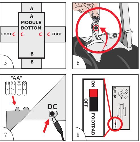
Insert 4 AA alkaline batteries (not included) into the 7. battery compartment located on the top of the MODULE or connect the DC Adapter (sold separately).
